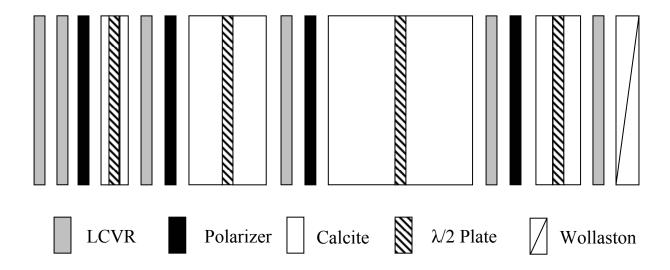
Figure 3. Diagram of the optical components of the filter/polarimeter. The identification of the elements is indicated below. Light enters from the left. Dimensions are not to scale, except for relative thicknesses of calcite elements.
